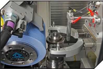
Tremec's dual-clutch transmission development utilizes Klingelberg's Speed Viper gear grinding technology. The two companies have collaborated on projects since 1993. This case study examines the advantages of closed-loop technology.
