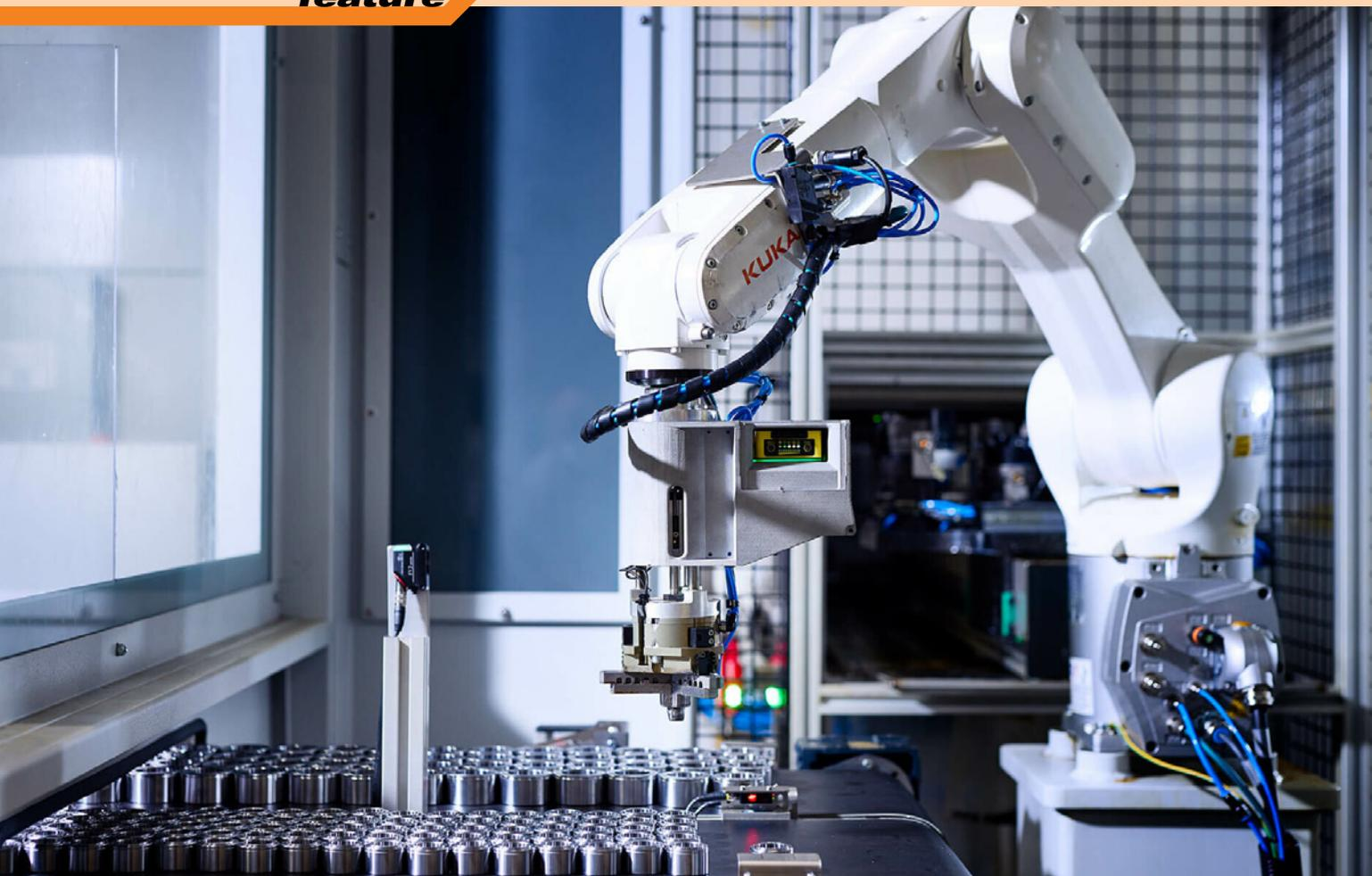
Figure 4—Industrial robots combined with the latest 2D/3D sensor technology for capturing the position of components will be key to flexible automation in the future.
