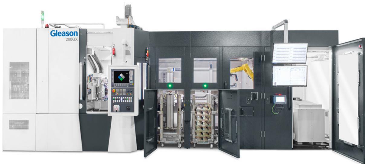
The stacking cell accommodates baskets of various manufacturers and styles and is ideally suited for the autonomous processing of large lot sizes of gears.
