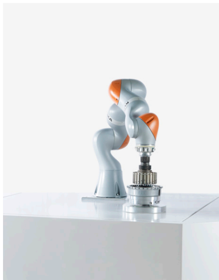
With its integrated torque sensors, the KUKA LBR iiwa enables the automation of delicate assembly tasks for force-controlled joining operations and process monitoring.
