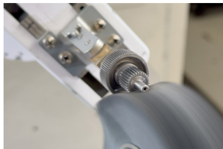
A cluster gear at the second Scotch-Brite wheel.
