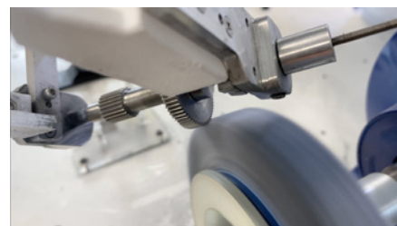
A cluster gear mid-cycle, seen from below. The OB7’s seventh axis allows compound approach angles that a 6-axis arm can’t reach.
