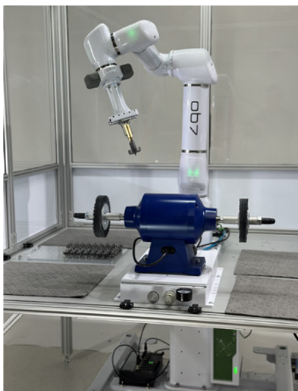
Inside the enclosed cell, the OB7 holds a part between dual deburring wheels. The offset and pressure adjustment dials are visible on the platform base.
