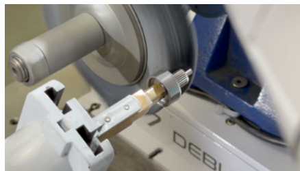
A pinion shaft held by custom gripper fingers approaches the finishing wheel.
