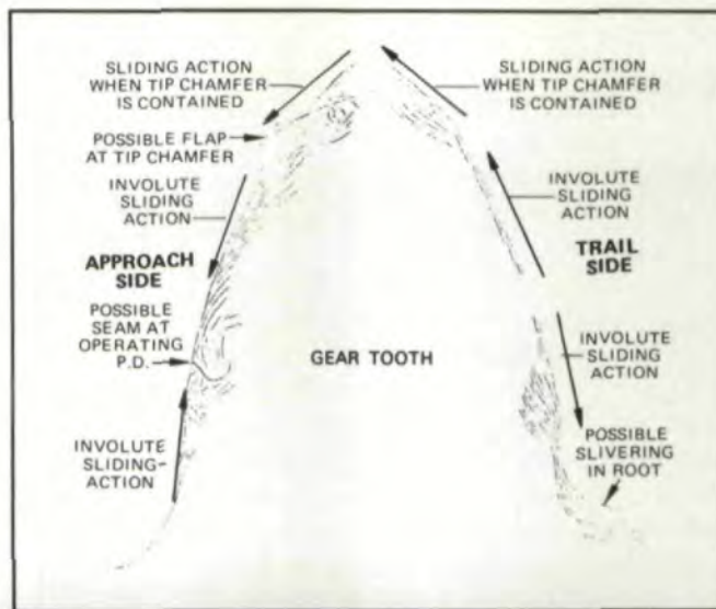
Fig. 5 (right) — Tooth flow pattern that results when too much stock is left for roll-finishing, or when material hardness is excessive.
