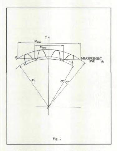
restriction for the maximum allowable amount of span measurement:
