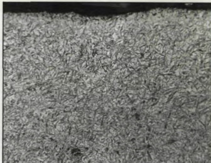
Fig. 9b — Cr-free root area surface. Structure is martensite and austenite. (400X)
