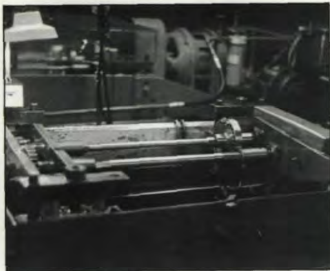
Fig. 1 — Power circulating gear test rig. Test gears are on the left.
