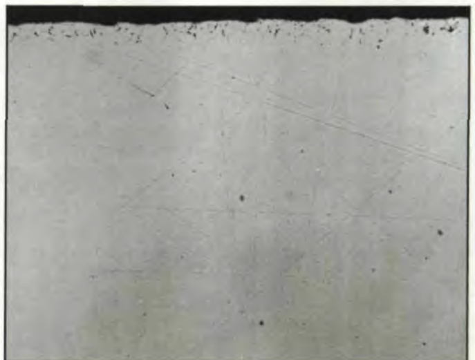
Fig. 8b—(Cr-Free) Flank surface (unetched showing IGO penetration (0.0007).
