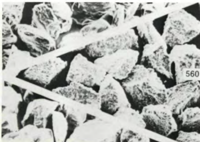
Fig. 2—Typical crystals of cubic boron nitride.
