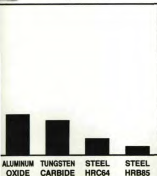
Fig. 1—Hardness comparison of typical materials.
