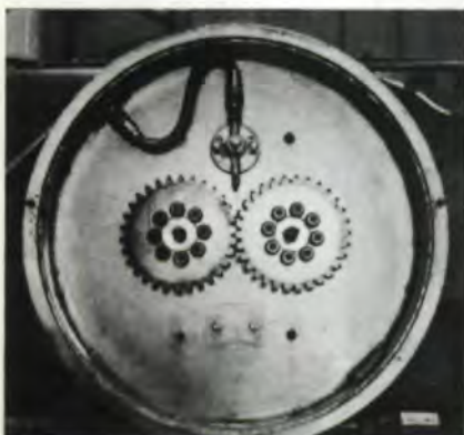
Fig. 13—Rig for rotating surface durability and scoring test.
