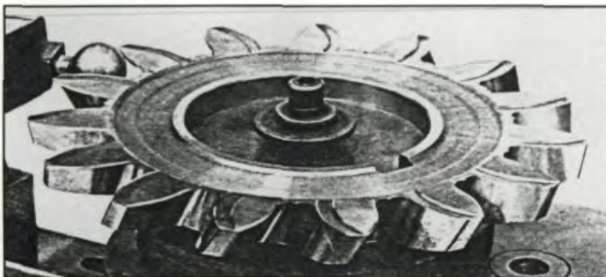
Fig. 2-20 – Groove and lip sharpening on herringbone cutter.
