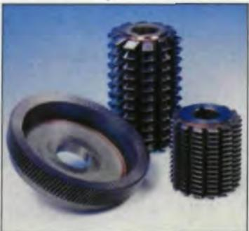
The outstanding high performance of Balzers TiCN coating can clearly be seen in the gear cutting example shown here. As significant is the performance of the reground tool without the need to recoat.
