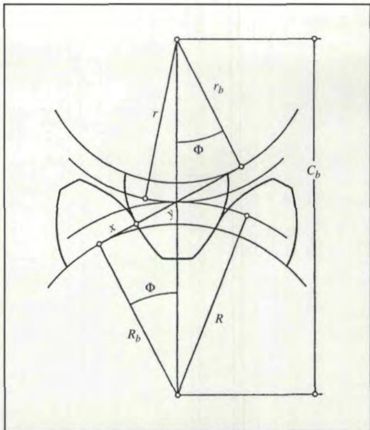
Fig. 1 — Reference circles and tooth profiles in contact.
