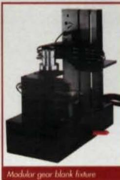
Modular gear blank fixture
