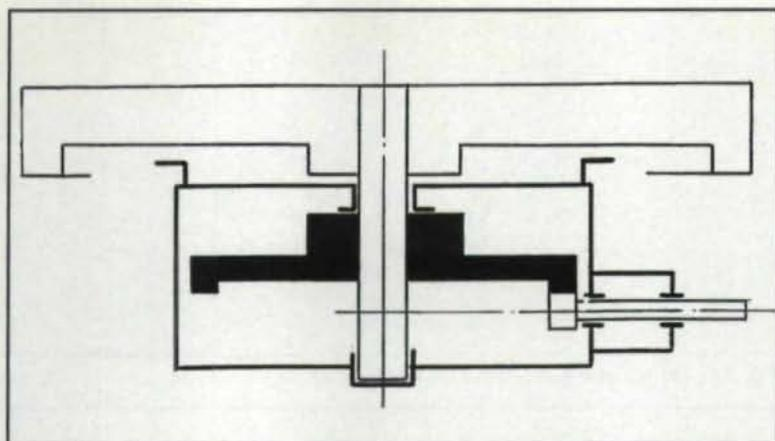
Fig. 5 — Single-stage driven turntable ( $i = 10$ ).
