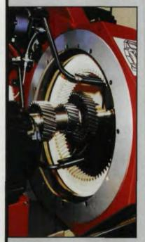
Fast, economical hard gear finishing process that increases gear life while reducing or eliminating gear noise.
