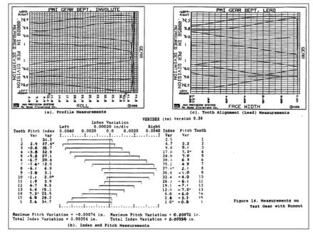
Looking at the characteristic of the traces can be useful when determining what to fix in bringing the gear within tolerance.
