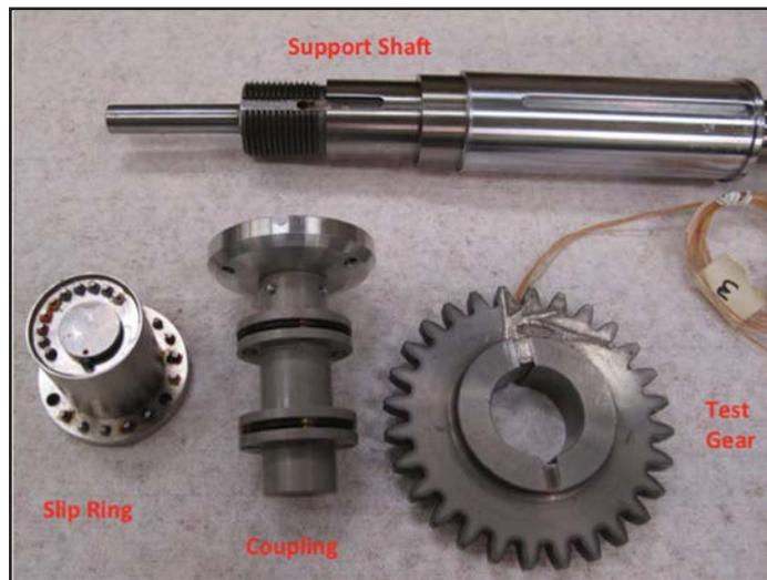
Figure 11 Loss-of-lubrication test specimen and related components.
