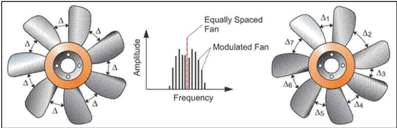
Figure 1 Cooling fan with unequally spaced blades.
