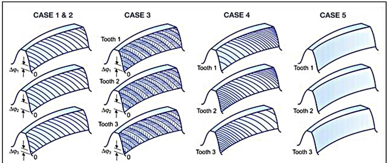
Figure 2 Tooth mesh surface structure and excitation change.
