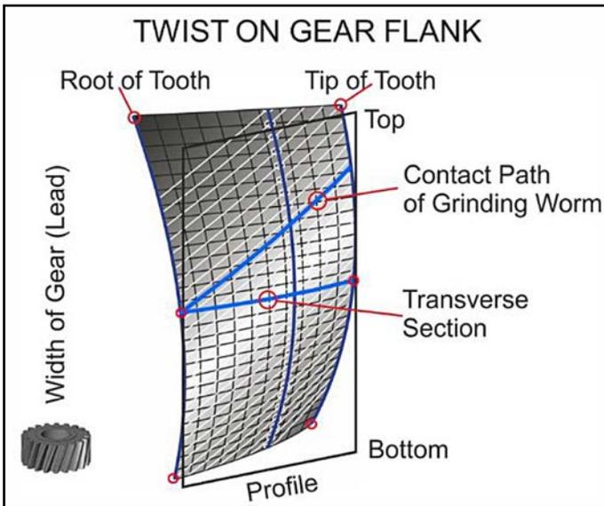
Figure 4 Flank twist.
