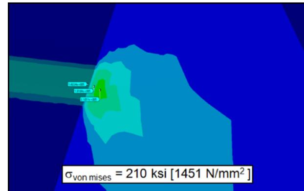
Figure 15 Preload operation von Mises stress.
