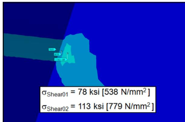
Figure 13 Preload operation shear stress.
