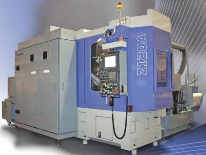
The world's only threaded wheel grinder for internal gears is a technical triumph: the ZI20A. Designed for quieter automobiles - EV, HEV and conventional planetary transmissions, it allows customers to accurately and quickly hard finish internally toothed ring gears — at significantly lower production costs.
