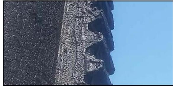
Figure 20 Greased rack for operation.
