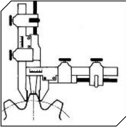
**Figure 3** Chordal measurement from AGMA 2002-C16, Figure 21.
