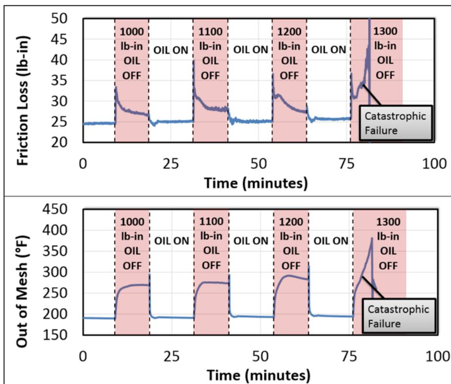
Figure 9 Load step searching test.
