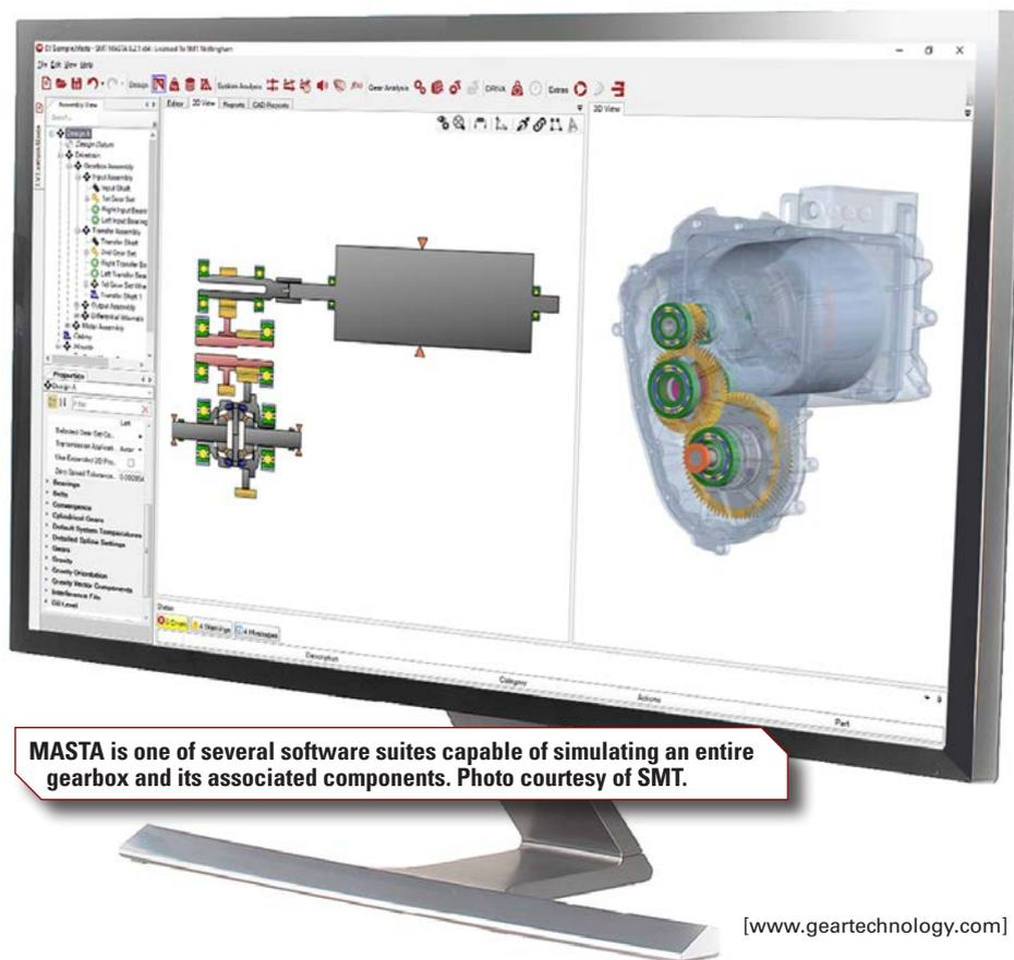
**MASTA is one of several software suites capable of simulating an entire gearbox and its associated components. Photo courtesy of SMT.**
