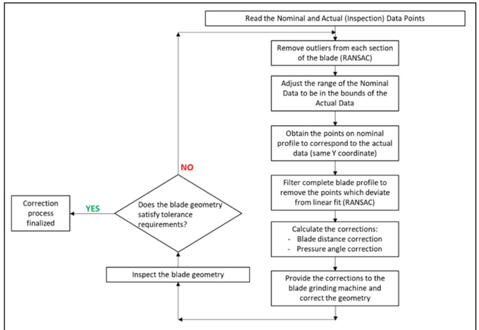
Figure 11 Summary of the proposed procedure for blade correction.
