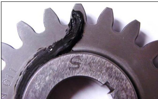
Figure 12 Thermocouple instrumented gear.
