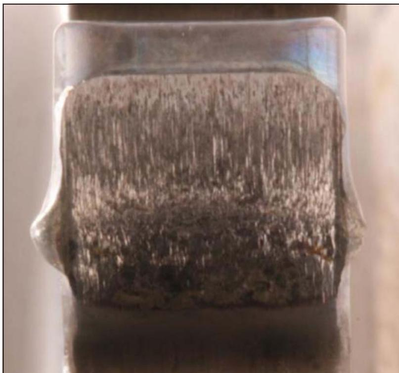
Figure 8 Catastrophic failure, stopped prior to loss of power transmission.
