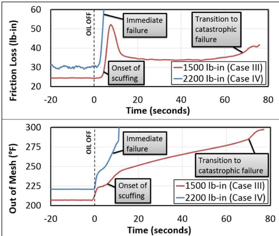
Figure 6 Case III vs. Case IV severity comparison.
