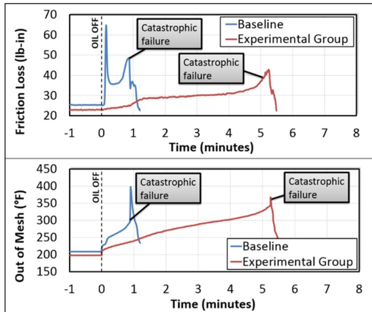
**Figure 15** Experimental vs. baseline performance comparison.
