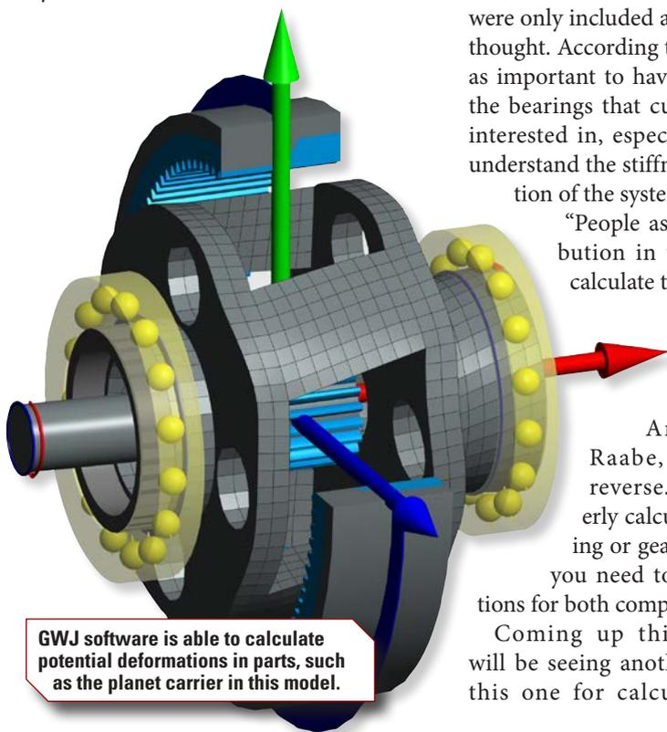
GWJ software is able to calculate potential deformations in parts, such as the planet carrier in this model.
