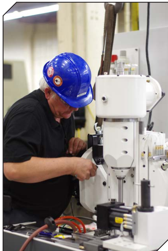
Billy Rodgers (a lead gear machine builder at Bourn and Koch) assembling a B&K 100H gear hobber.
