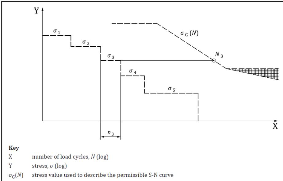
**Figure 7** Stress spectrum and S-N curve, Figure 3 in ISO 6336-6:2019. The figure explains how for a given stress level  $\sigma_i$ , an allowable number of load cycles  $N_i$  can be determined using the S-N curve(s) determined along ISO 6336-2 and -3. Note that the value  $\sigma_G$  is either  $\sigma_{HG}$  or  $\sigma_{FG}$ . Above two figures were combined in one figure in 2006 edition, lacking some clarity.
