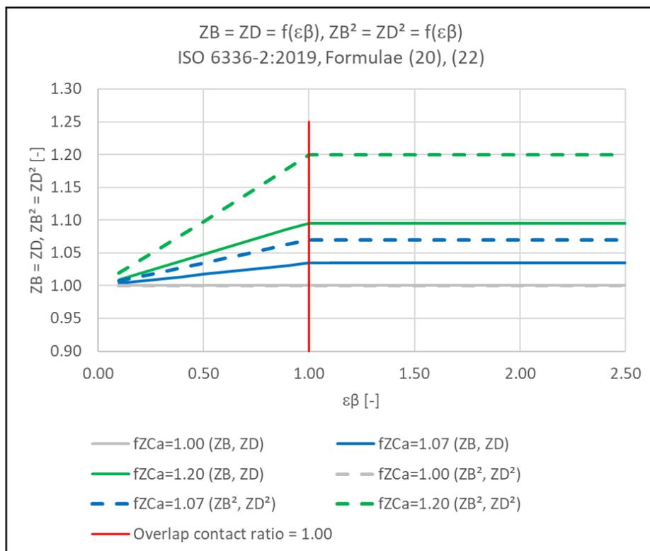
Figure 2 Zone factors  $Z_{K_{H\beta-C}} B$  and  $Z_D$  and their square as a function of  $f_{ZCa}$  and overlap contact ratio  $\epsilon_\beta$ .
