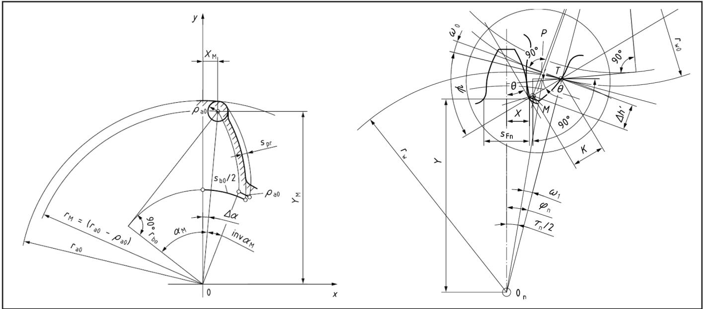
**Figure 4** Left: Quantities at the shaper cutter, (Ref. 6). Right: External gear in mesh with shaper cutter, coordinates  $X$  and  $Y$  of tangent point, tangent angle  $\theta$  and tooth thickness  $s_{Fn}$ , (Ref. 6). Tooth root fillet radius  $\rho_F$  and the bending moment arm  $h_{Fe}$  not shown explicitly.
