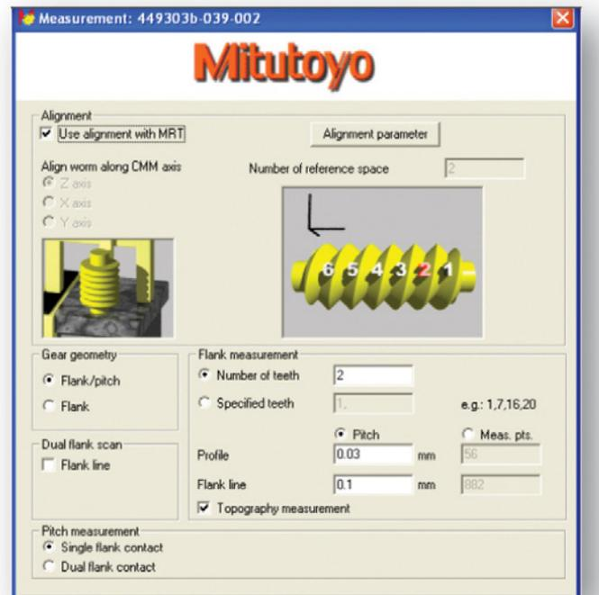
Special CMM software supports measuring several types of worm gears using a touch trigger probe or scanning probe on a CMM.
