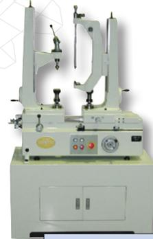
GTR25 Double Flank Gear Roller
