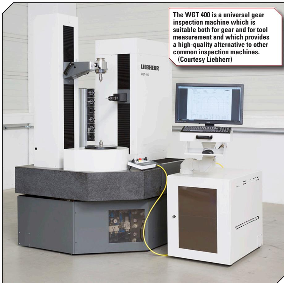
**The WGT 400 is a universal gear inspection machine which is suitable both for gear and for tool measurement and which provides a high-quality alternative to other common inspection machines. (Courtesy Liebherr)**
