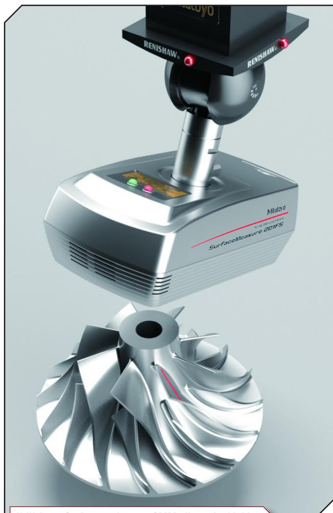
Utilizing a Surfest probe on a CMM allows for highly accurate measurements of complex parts, including gears and impellers.
