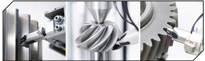
Figure 10 Magnetic Barkhausen noise analysis is an alternative to detect grinding burn.
