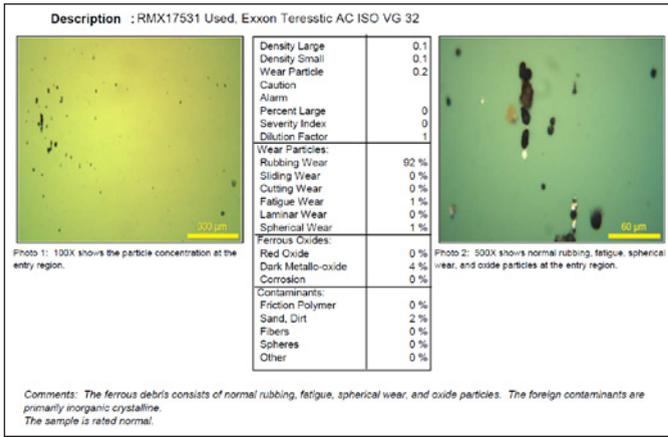
Figure 2—Analytical ferrography of used lubricant. (Photo courtesy of Artec Machine Systems.)
