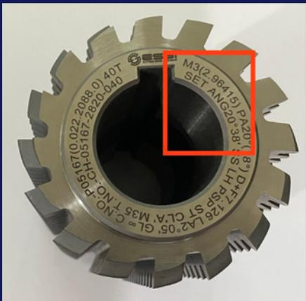
Figure 4—Hob marking for helical gear.
