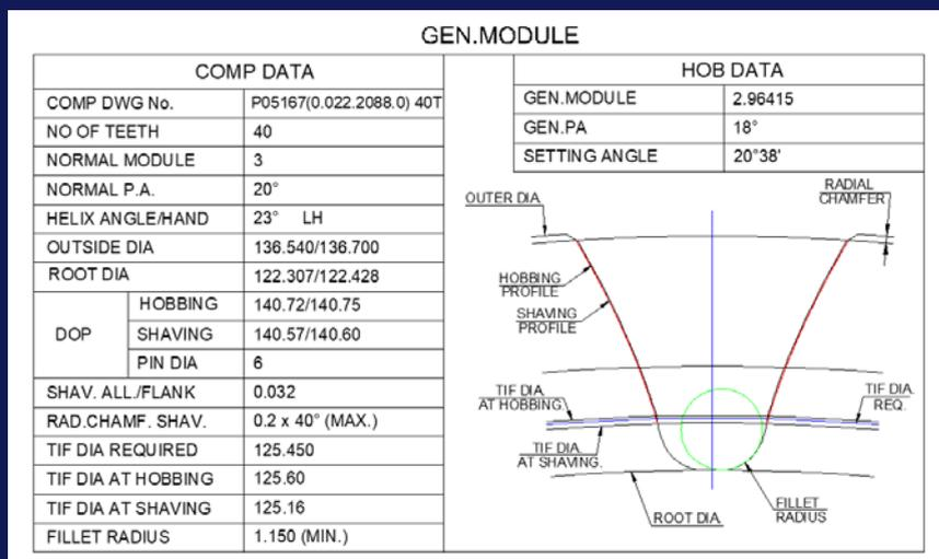
Figure 2—Component generated profile with corrected design.
