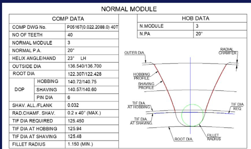
Figure 1—Component generated profile with standard design.
