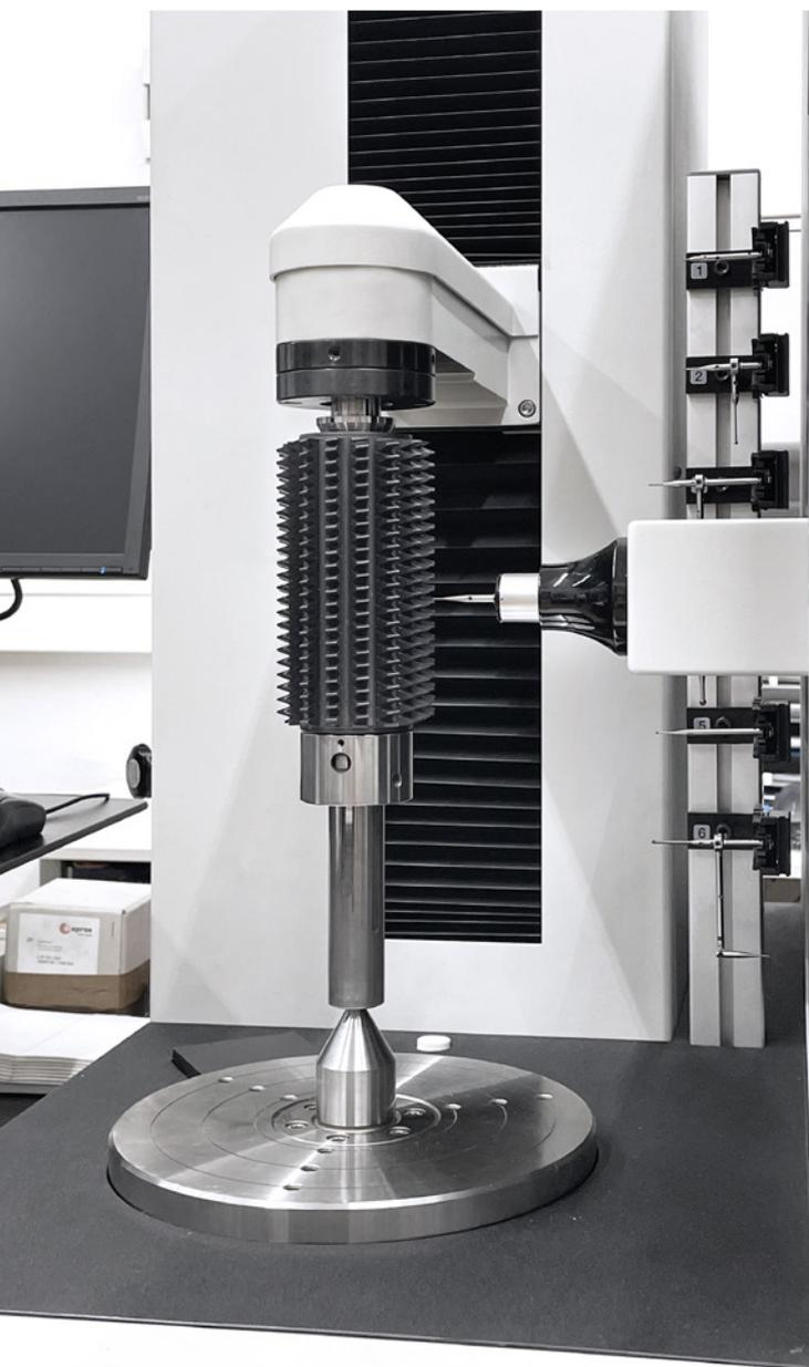
*The LeCount Type H model, with its extra-long jaws and narrow expansion range, is well-suited for the requirements of hob inspection. Additionally, the series offers spline mandrels, since not every part has smooth bores.*
