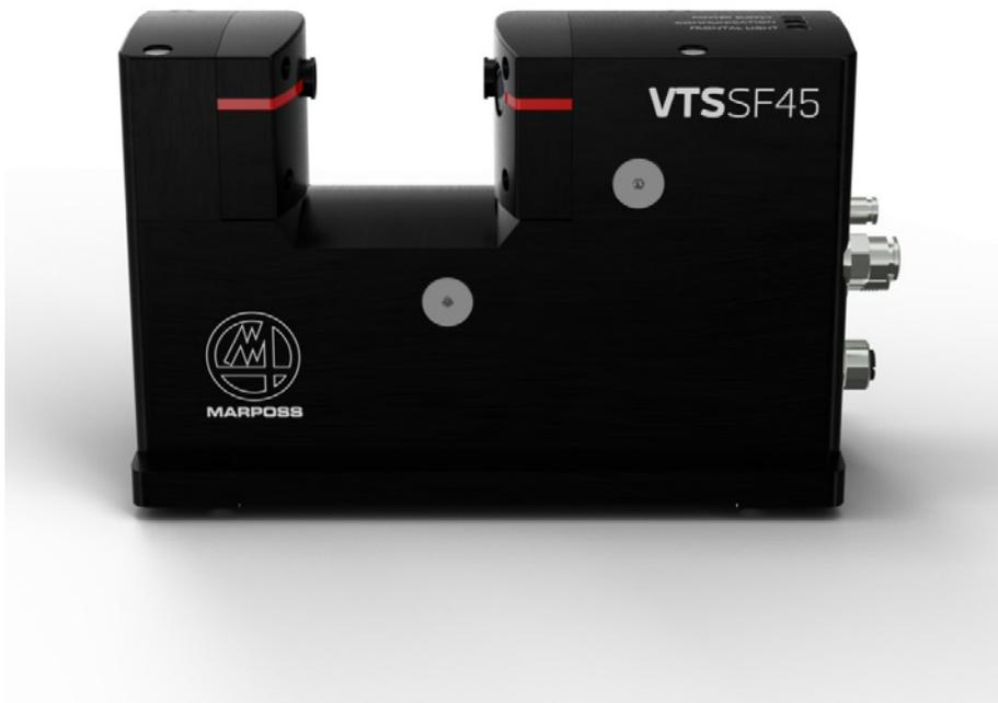
working spaces such as micromachining, semiconductor or moldmaking applications. The VTS SF-45 units are installed inside the machine working area to monitor actual tool working conditions without any contact while the tool can rotate at full spindle speed (up to 80k rpm) during data acquisition. Since there is no need to slow the spindle, presetting time can be reduced and measurement accuracy is increased to better eliminate collision hazards.
