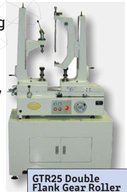
GTR25 Double Flank Gear Roller
