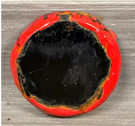
Figure 15—Test coupon F2703 after 1,341 hours of salt fog exposure.
