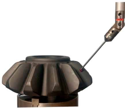
Figure 9—CMM evaluation and inspection report.
