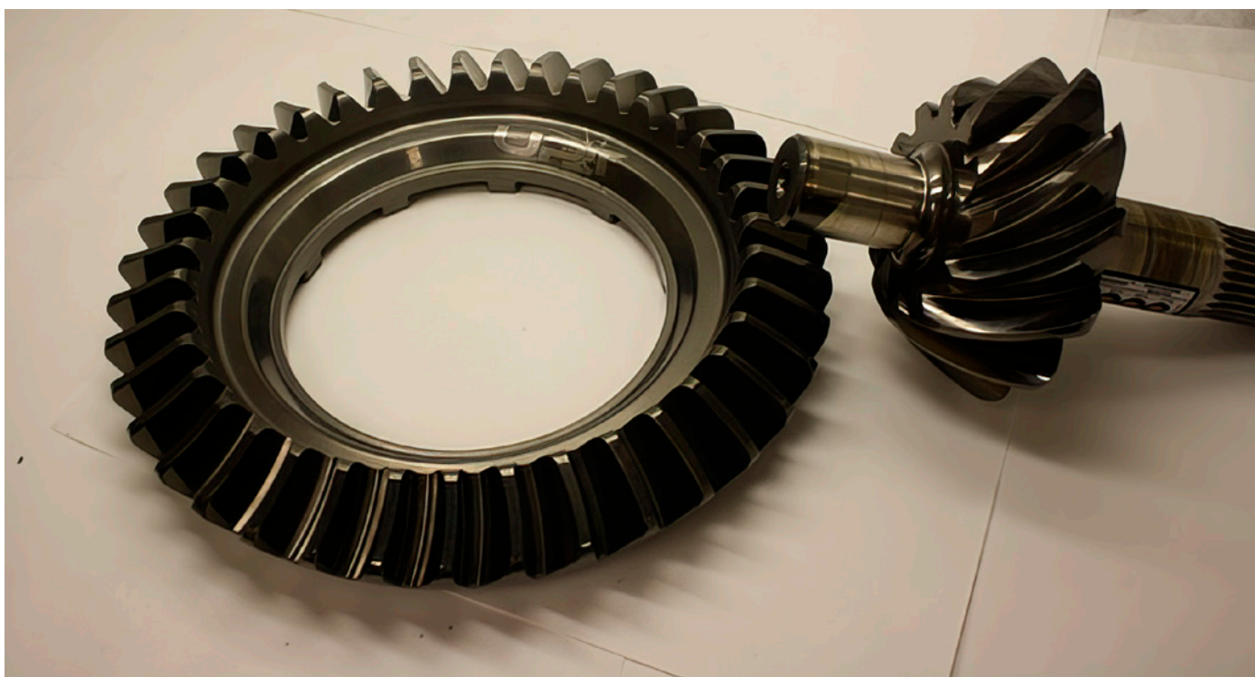
Figure 24—Ring gear and pinion from a competitive racing team, coated with the predecessor of the P51M coating system.
