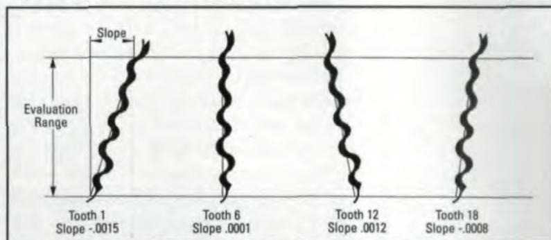
Fig. 3—Excessive slope variation can result from a fixture or blank runout.
