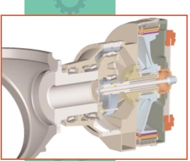
Five Feet in Diameter— An internal double helical ring gear lays at the center of a prototype 1.5 MW wind turbine designed by Powertrain Engineers Inc., then manufactured by Brad Foote Gear Works Inc. of Cicero, Illinois.
