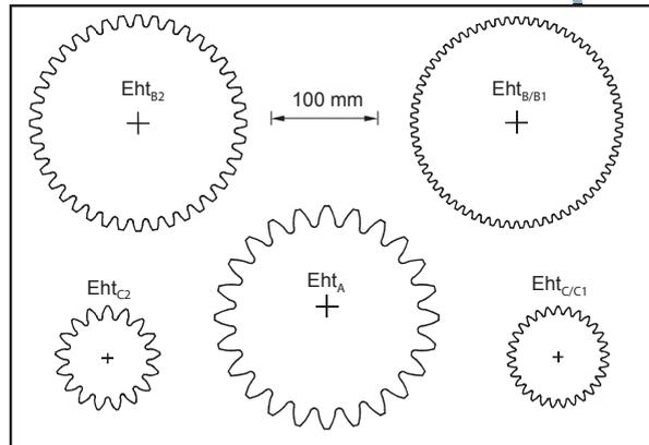
Figure 2—Gear types (pinion) of the test program.
