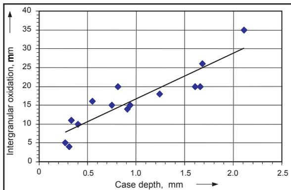
Figure 7—Case depth and intergranular oxidation of bending test gear types  $Eht_A, Eht_B, Eht_C$ .
