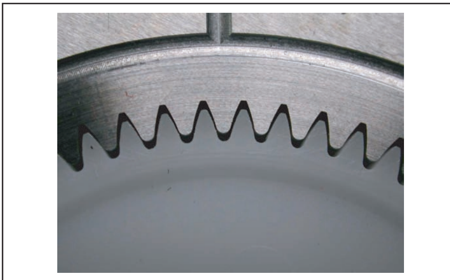
Figure 5—The involute shrinkage of a molded gear.
