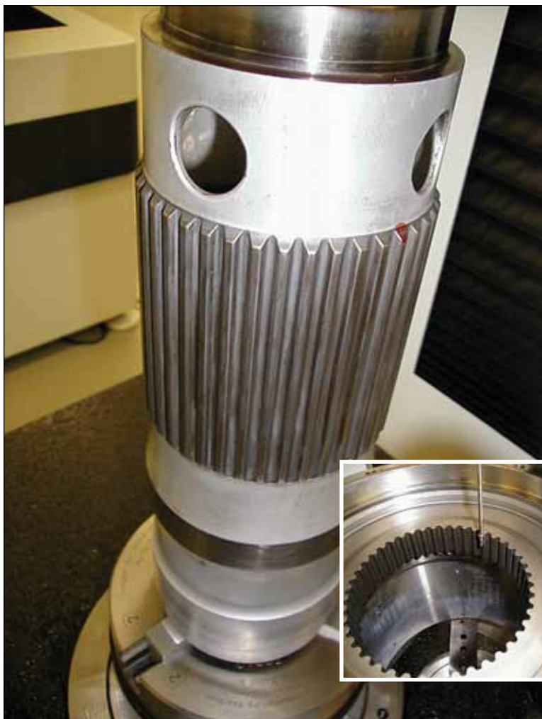
PECo's data acquisition and Renishaw 3-D probe technology enables the machine to generate measurements on various surfaces (All photos courtesy of PECo).
