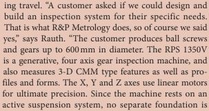
required. The high precision, air bearing rotary table is mounted on a granite bed and is driven directly by a torque motor." The RPS 1350V achieves the highest European class for inspection equipment accuracy: VDI/VDE 2612/13 Group I. Using an industry standard CNC control system, the RPS 1350V is I++ compliant, allowing the use of many CMM inspection packages.
