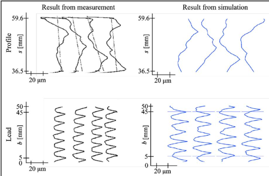
**Figure 8** Inspection chart over profile and lead for a gear; hobbed at the feed rate  $S=8.0$  mm/rev. On the left, results from industrial hobbing machine; and right, results from simulation are presented.
