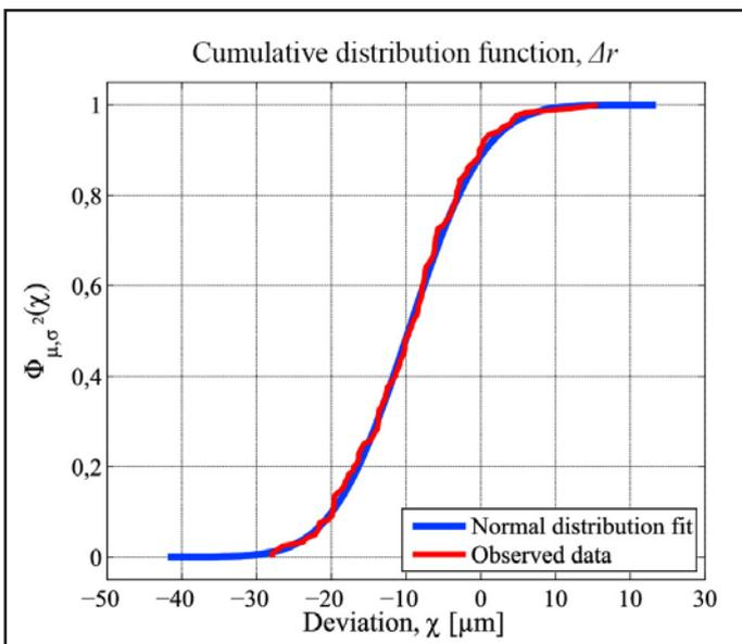
Figure 2 CDF: plot, radial deviation of inserts.
