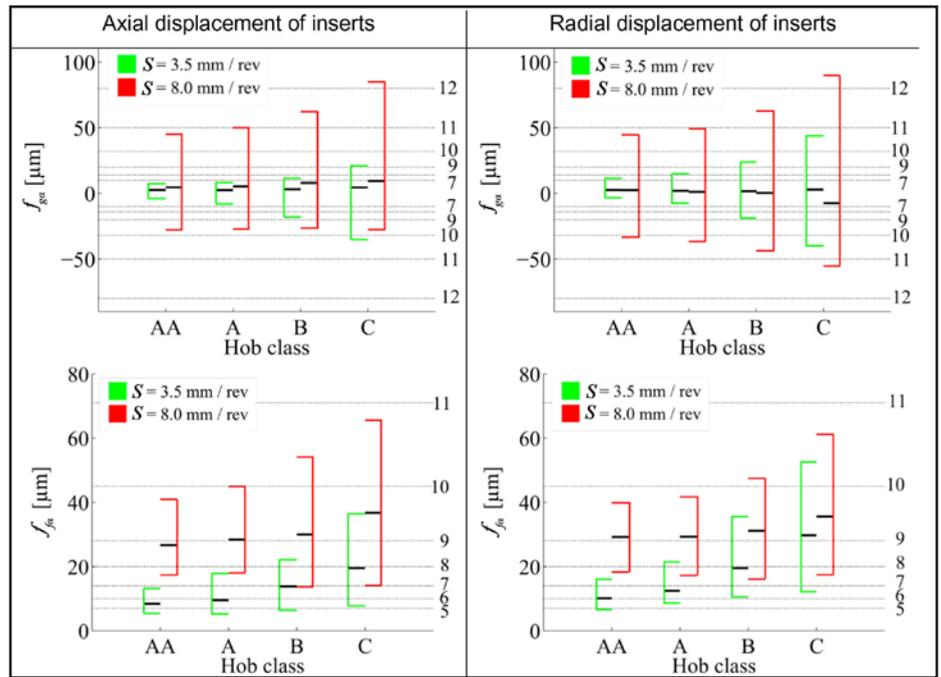
**Figure 6** Result from simulation where the profile deviations are plotted with varying hob classes. On the left ordinate, the gear tooth deviation, and on the right ordinate, the gear quality, is plotted.
