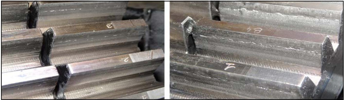
**Figure 18** Tooth flank after 10 Mcycles at 1200 MPa.
