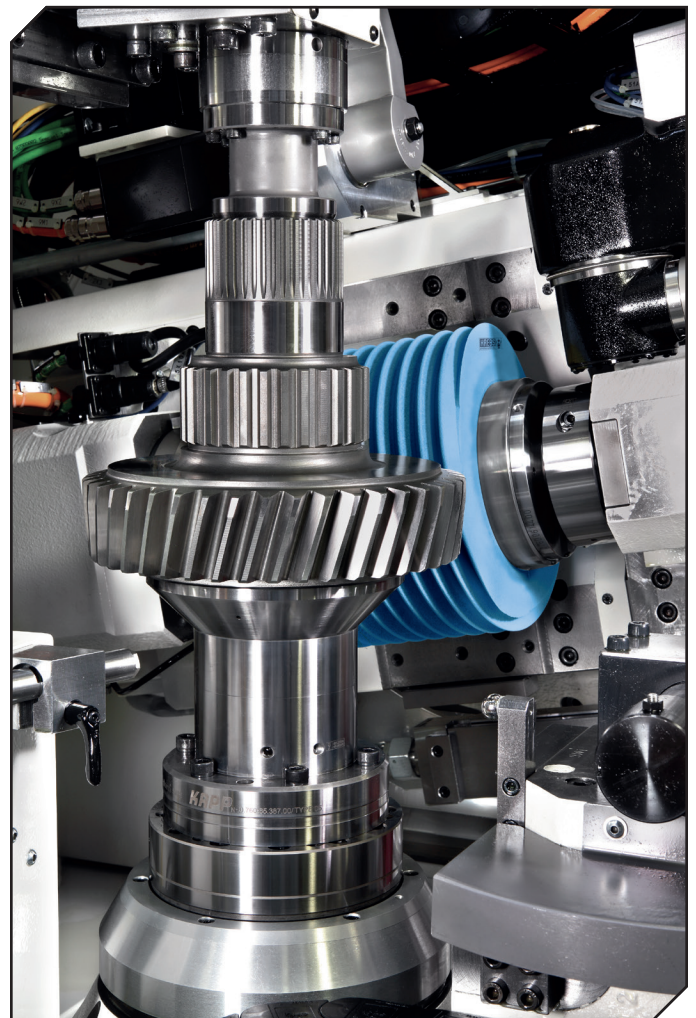
Continuous generating grinding with fine and polishing zone. Picture copyright: Kapp-Niles.
