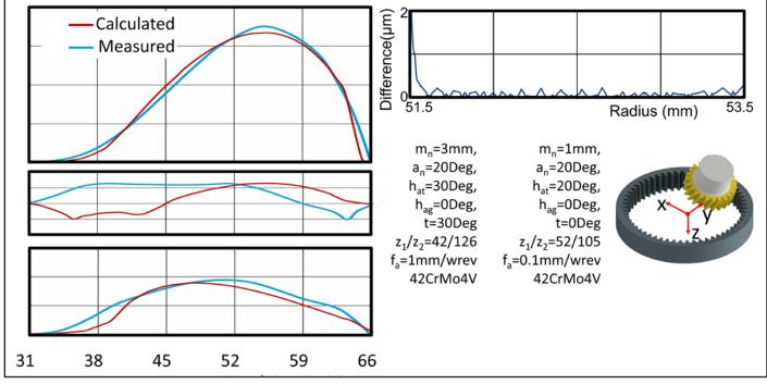
Figure 5 Cutting force (left) and surface topography validation (right).
