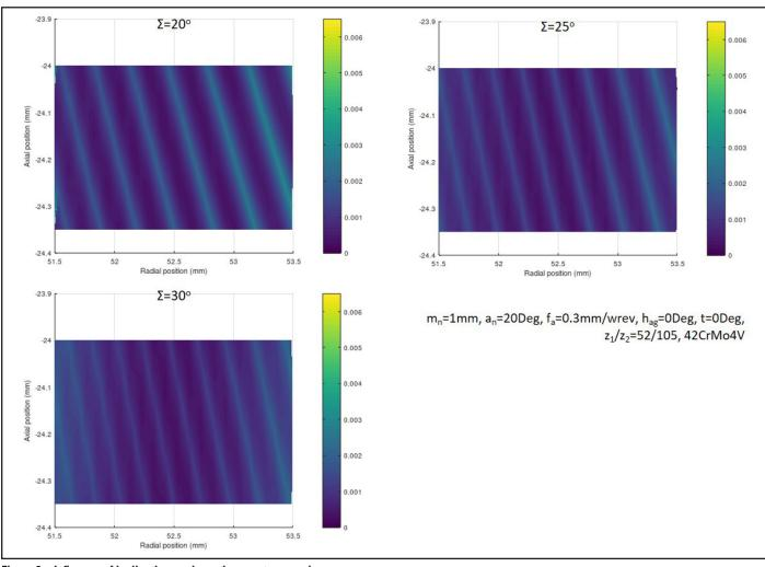
Figure 8 Influence of inclination angle on the gear topography.
