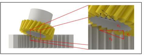
Figure 2 Cutting velocities during gear skiving ( $v_1$  rotation of the work gear,  $v_2$  rotation of the tool,  $v_c$  resulting cutting speed).
