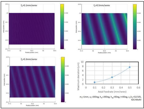
Figure 7 Influence of feed rate  $(f_a)$  on the gear topography.
