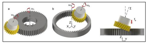
Figure 1 Gear skiving process kinematics for internal (b) and external gears (a).
