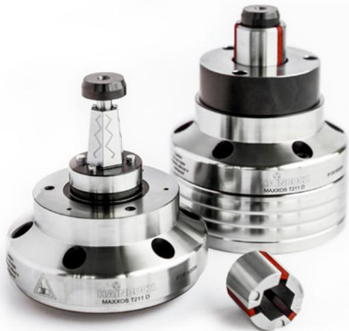
users can choose from up to three mandrel sizes depending on the clamping diameter. The larger the mandrel is, the greater its stability and rigidity. Smaller mandrels may be able to handle more of the customers smaller workpieces. The aligned, segmented clamping bushings have a minimum concentricity of 0.01 mm and can even be supplied in a high precision version.
