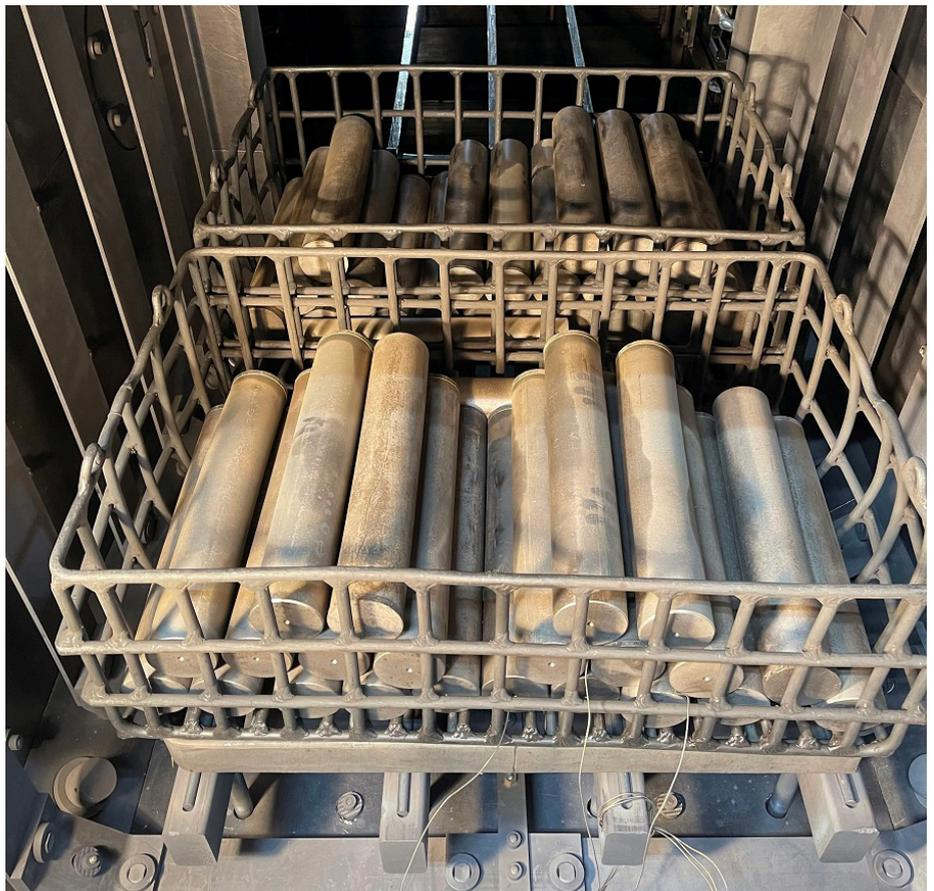
devoid of oxygen there is no need to use problematic oxygen probes. Material surfaces are free from intergranular oxidation (IGO) along with zero evidence of decarburized or carburized surface conditions. Heat treated components emerge from the quench oil bright and clean! With carbon potential issues totally eliminated, alloys of dissimilar carbon contents with comparable cross sections and austenitizing temperatures, can all be treated within the same load.
