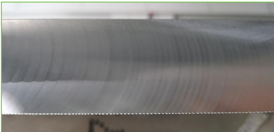
**Figure 5** With the optimum combination of cutting speed, feed rate and depth of cut, the robot produces better surfaces than required. Chatter marks remain absent.
