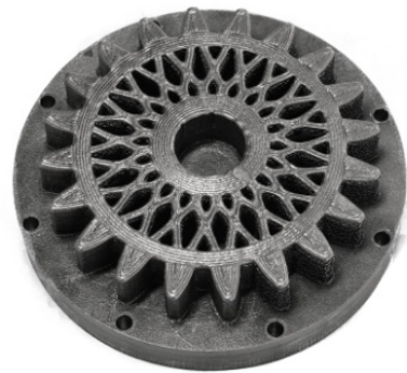
A LAMDA DED-printed gear made of AISI 304 stainless steel demonstrates lightweighting design potential.
