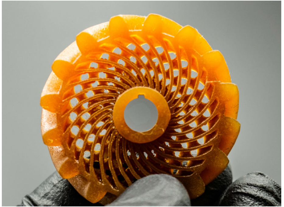
A 3D-printed gear made with Fortify's HTS resin.
