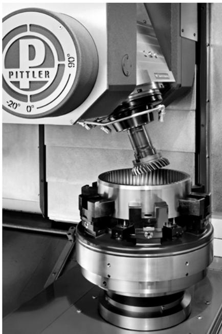
Figure 6—Skiving technology comparison. (Source: Pittler T&S)
