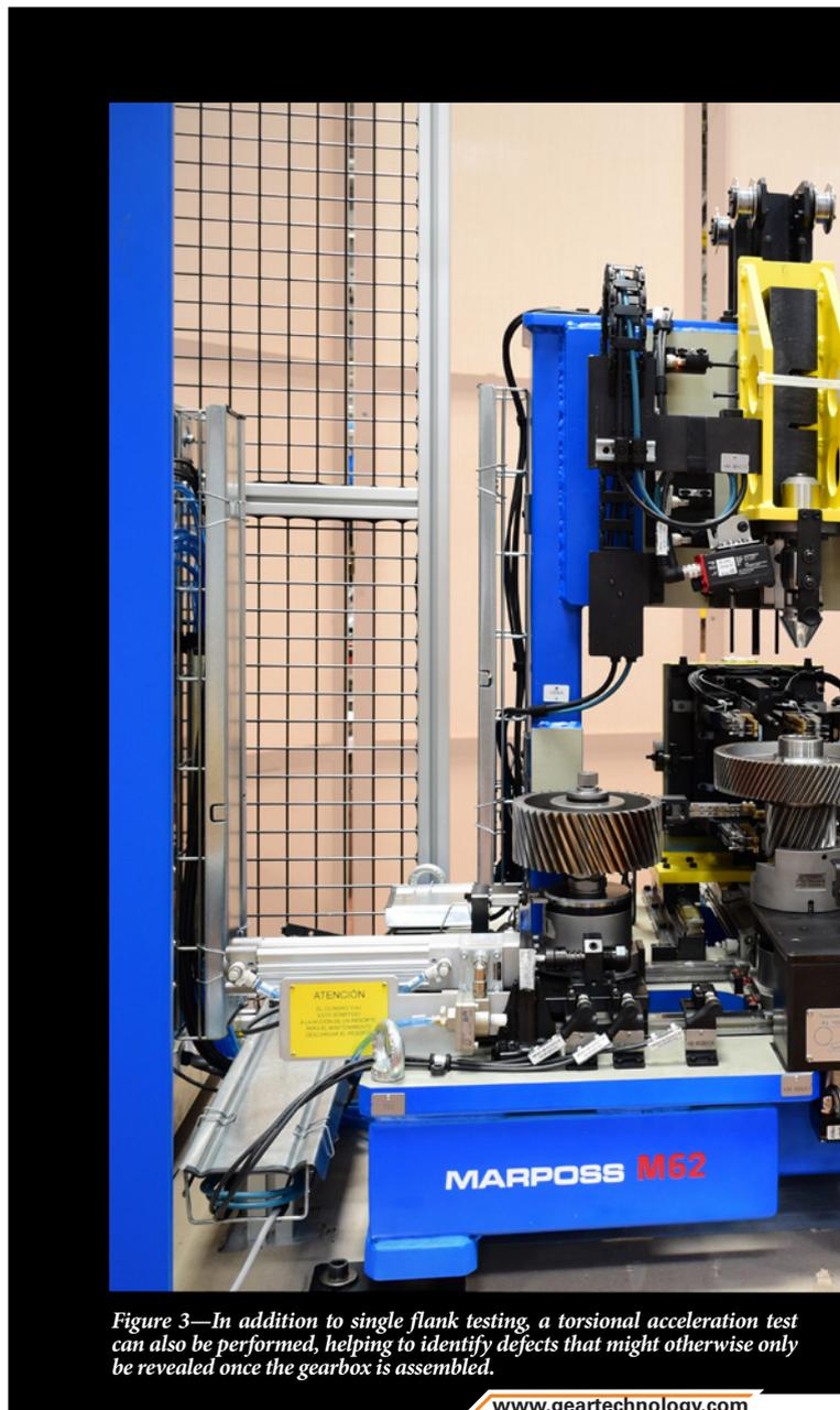
*Figure 3—In addition to single flank testing, a torsional acceleration test can also be performed, helping to identify defects that might otherwise only be revealed once the gearbox is assembled.*
