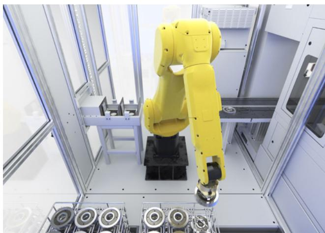
*Figure 3—In automation cells with basket stacks, the system is loaded and unloaded by baskets from which the robot picks up or deposits the oriented workpieces. The empty baskets are transferred to the stack by the robot.*
