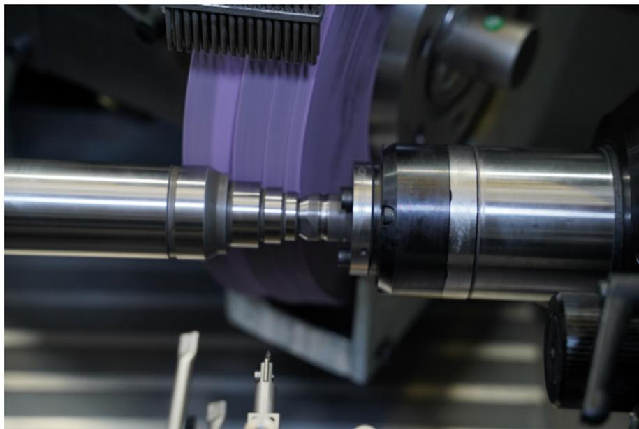
Figure 11—Grinding in single clamping. (Source: BUDERUS Schleiftechnik)
