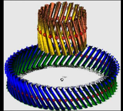
Figure 6—In Marposs' newest system laser profile sensors and the optical triangulation principle help reconstruct a 3D model of the component being measured.
