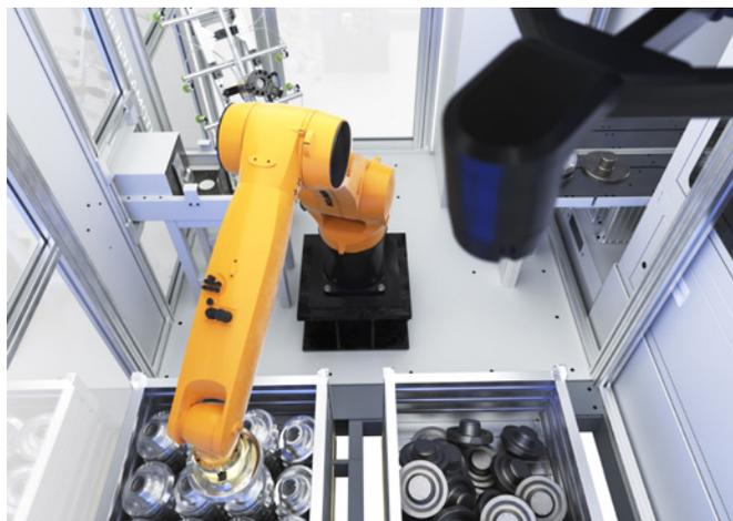
*Figure 2—In bin picking systems (“reach into the box”), the workpieces are in a chaotic position. With the help of a 3D sensor system, the robot not only picks the components but also correctly recognizes and aligns them and feeds them to the next processing step.*
