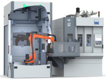
Figure 1—The equipment options of the individual robotic cell (here next to a VL 4) are large—from statistical process control (SPC) to deburring systems.
