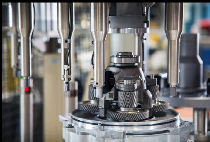
Figure 1—Gears for electric drives need to be designed with tighter manufacturing tolerances, especially around profile and lead features.
