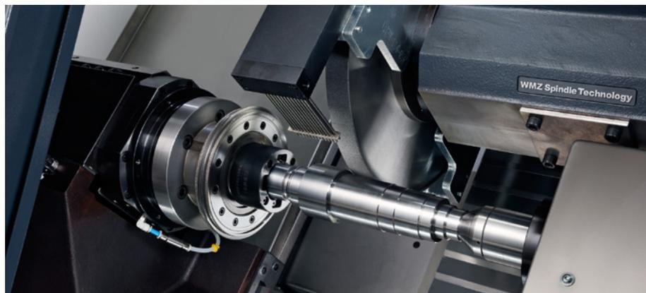
Figure 12—Grinding in single clamping with WMZ Spindle Technology. (Source: BUDERUS Schleiftechnik)
