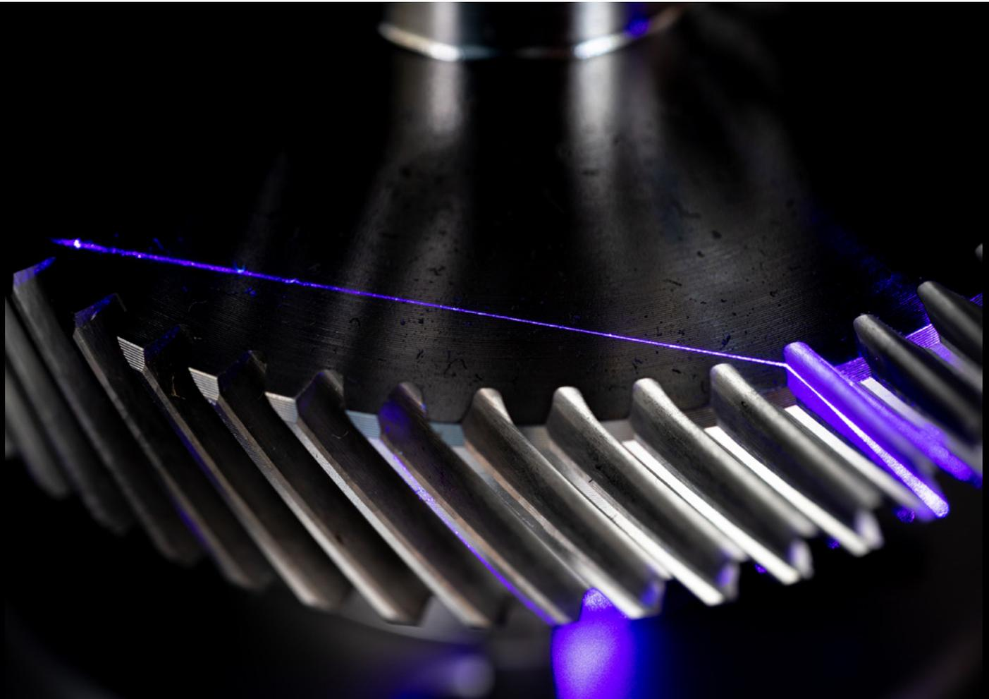
Figure 5—The application of noncontact technology—such as lasers and cameras—is also evolving to tackle the increased need for gear measuring in e-drives.
