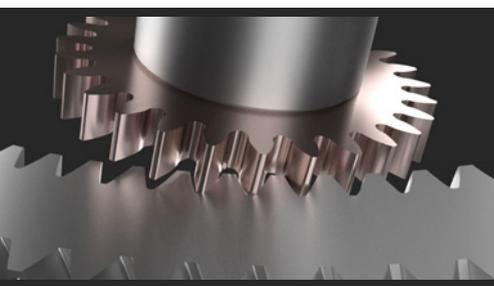
Figure 4—Animation of the skiving process. (Source: Pittler T&S)
