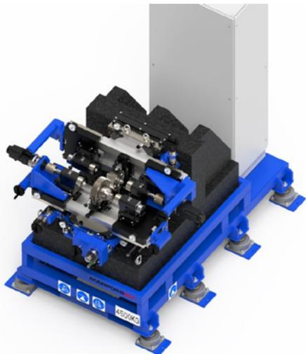
*Figure 2—This gear tester from Marposs works on the single flank testing method where a master gear meshes with the component under inspection, identifying defects not detectable with traditional production tests.*
