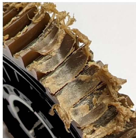
Figure 11—Thermal failure on the worm wheel run in dry, non-lubricated conditions.
