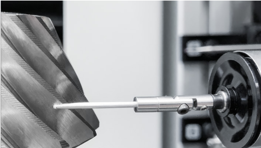
Figure 2—Skidless surface finish probe.
