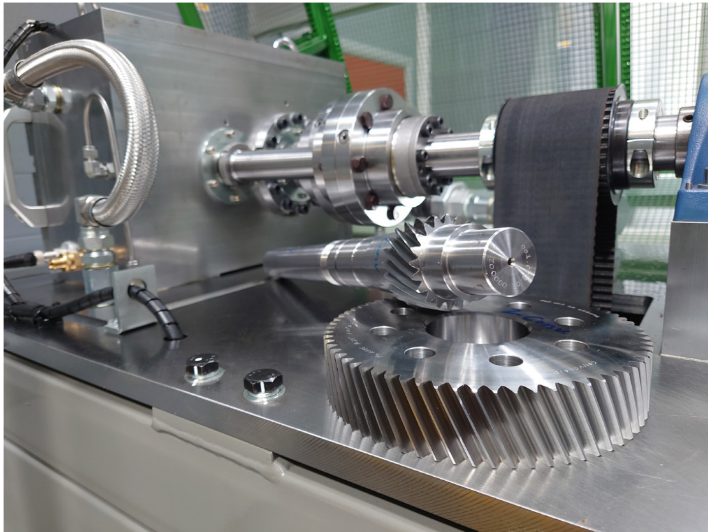
An in-house back-to-back rig built for non-involute gears. (All images: Dontyne)
