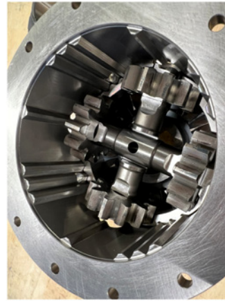
Figure 7—Photograph of a realized differential with crown gears.
