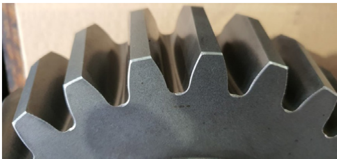
Figure 10—Fully rounded root at midface.
