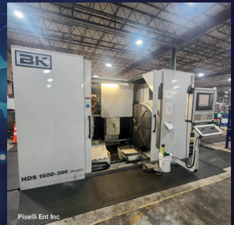
B+K CNC HORIZ GUIDELESS SHAPER HDS 1600 NEW 2011
