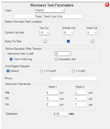
Figure 5—Shows an example of waviness programming within the GAMA interface.
