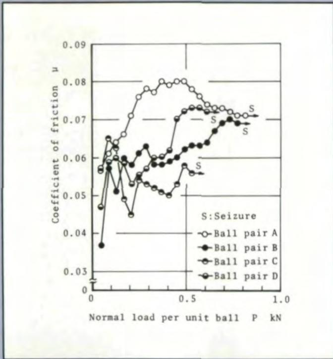
Fig. 4—Relation between coefficient of friction and load
