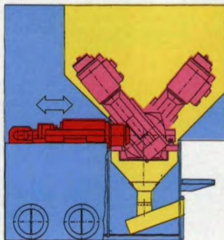
The entire work area is enclosed in a stainless steel shroud (yellow) that prevents hot chips from accumulating and directs them downward into a chip conveyor. Horizontal orientation of work spindle (red) helps facilitate chip removal.
