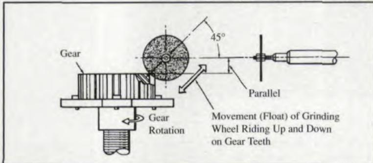
Fig. 4 — Alignment of grinding wheel.
