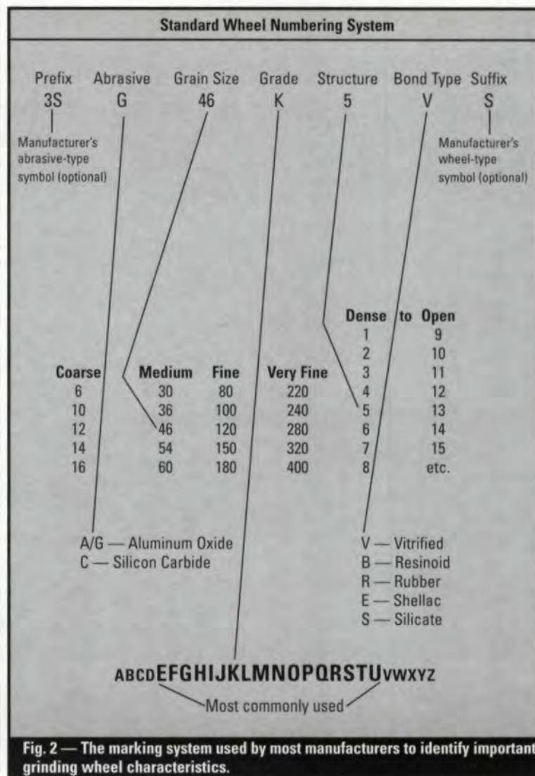
Fig. 2 — The marking system used by most manufacturers to identify important grinding wheel characteristics.
