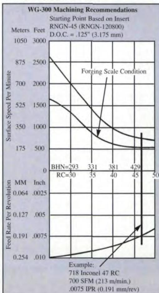
Fig. 5 — Sample nomogram for nickel alloy aircraft engines.
