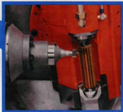
■ **Designed for dry.** The Pfauter P100 is a true dry carbide hobbing machine. The horizontal work spindle facilitates chip removal; and a work area completely enclosed in a stainless steel shroud directs chips downward and completely away from the work area. There's simply no place for "hot" chips to accumulate in a dry operation—the P100 is thermally stable!
