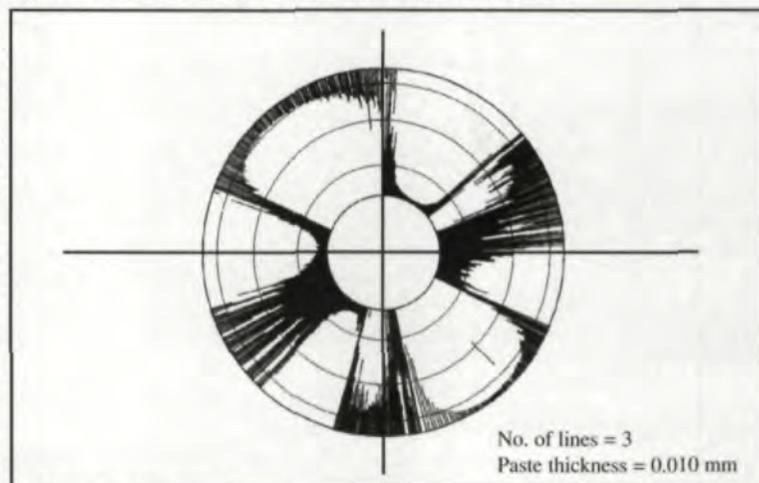
Fig. 4 — Bearing pattern for cylinder curve.
