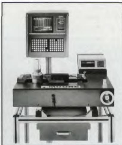
**Adjustable Pitch Diameter Inspection Gage**
