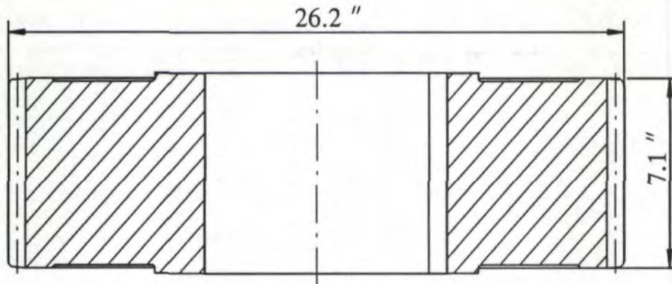
Gear for wind turbine drive system.
