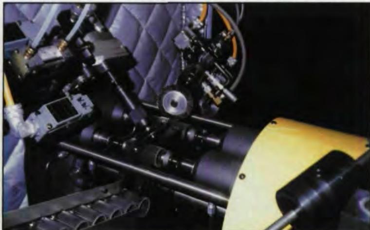
Fig. 1 — Deburring a helical pinion gear with power brushes.
