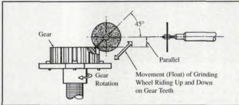
Fig. 4 — Alignment of grinding wheel.
