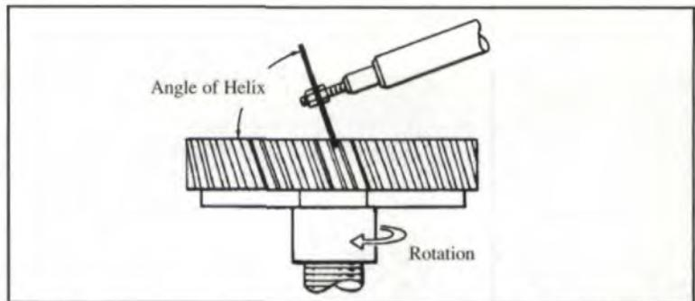
Fig. 8 — The grinding wheel angle must match the helix angle of the gear tooth.
