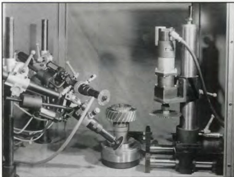
Fig. 3 — Removing exit burrs with a skiving unit and a grinding wheel.
