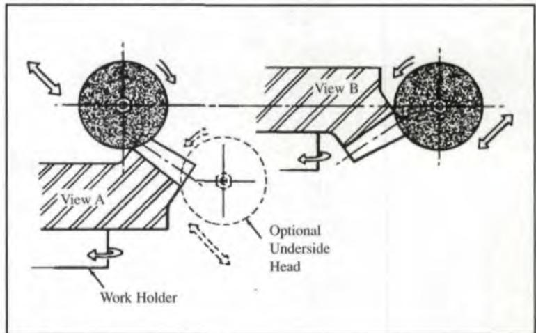
Fig. 10 — Straight bevel gear setup.
