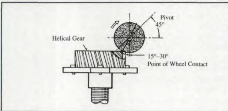
Fig. 6 — Helical gear wheel contact.
