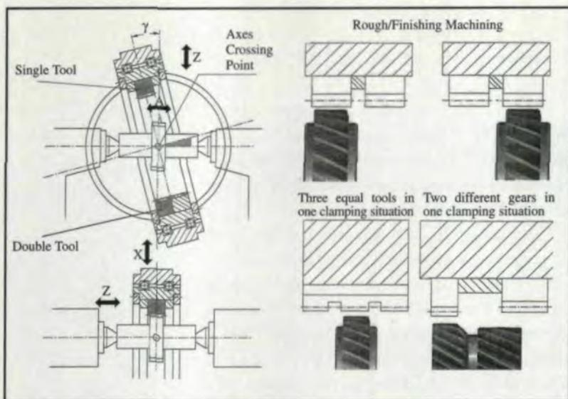
Fig. 6 — Advantages of the compound slide technique.
