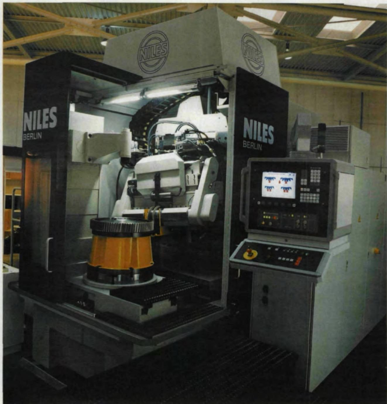
**The efficient solution for Gear Grinding up to 4,000 mm**
