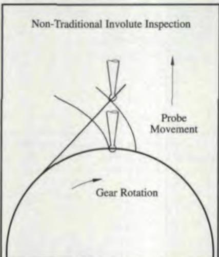
Fig. 5 — Mechanics of non-traditional involute inspection.
