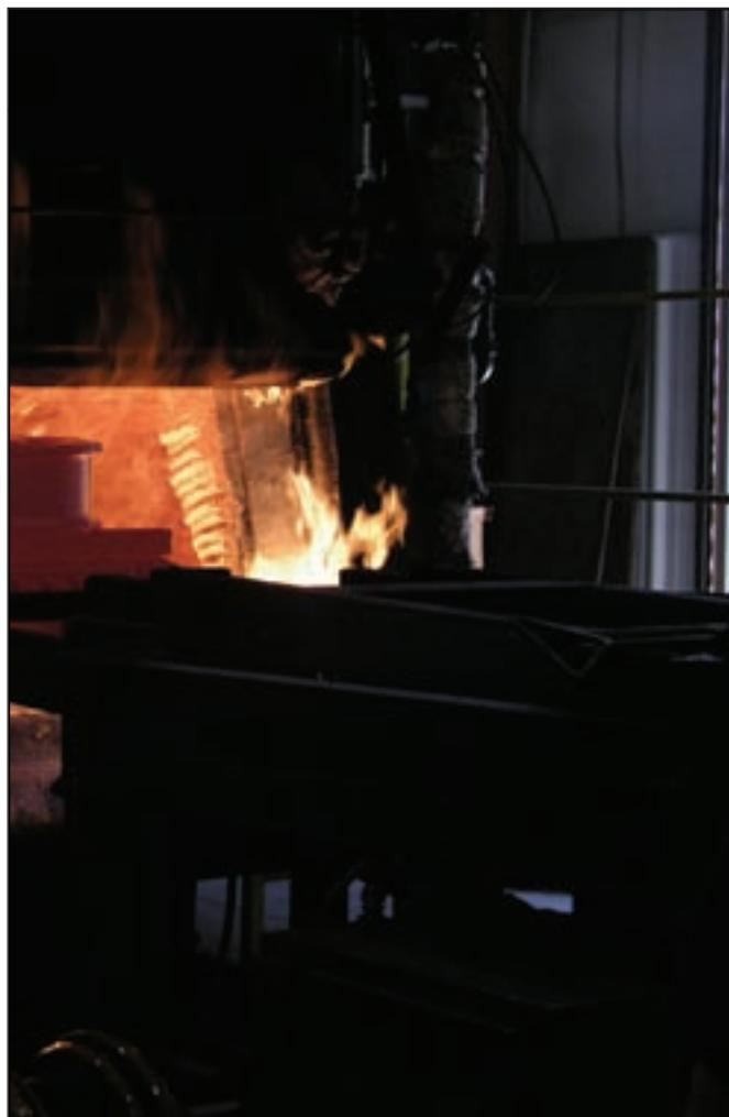
Upon completion, a heat treated wheel is pulled from the furnace at Xtek.
