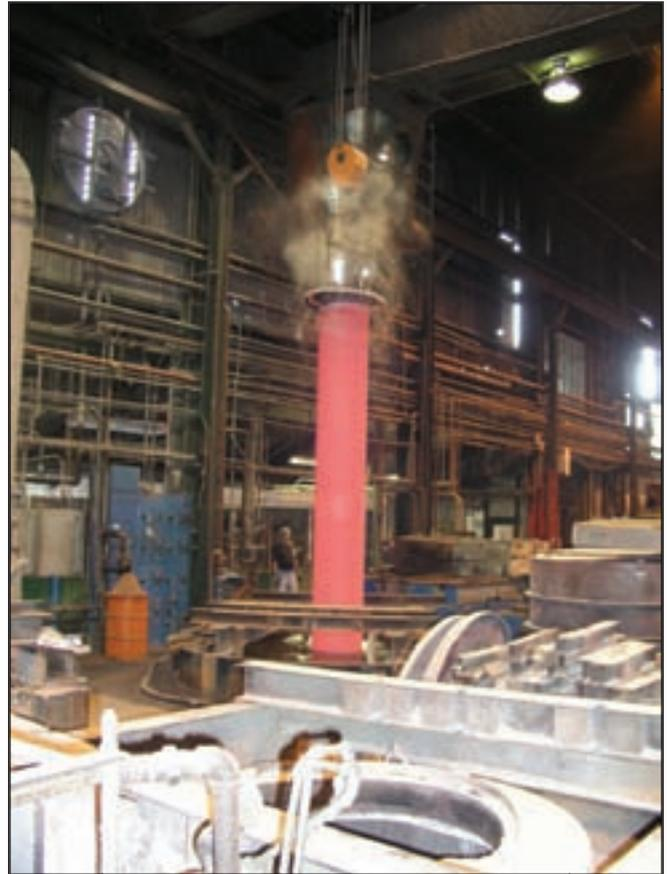
An in-process rope drum quenching at Xtek.
