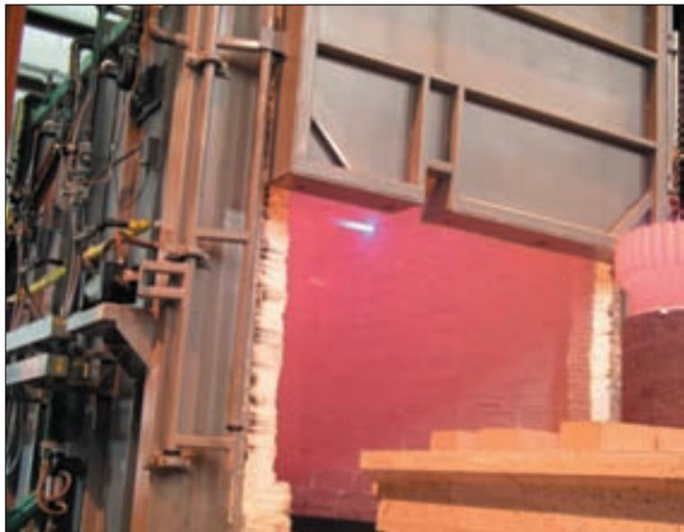
Xtek specializes in carburizing heavy equipment gears for its customers.
