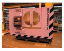
cylindrical blanks or shafts. A standard model features a NUM 1060H CNC control, tail center with variable load control, and it can hob wet or dry.
