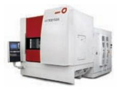
The NILES ZE 400 machine will also be at the Kapp booth, which has been one of the company's best selling products. The bed casting of the NILES ZE 400 is fashioned from thermally-optimized ductile iron to support a maximum workpiece weighing 2,650 pounds. The machine includes tailstock, CNC dressing device, on-board measuring and a Siemens 840D control. Siemens 611D simo-drives run the
