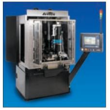
A servo-controlled stroking drive responds smoothly to the control's motion profiles. This feature provides the capability to perform conventional honing and single-pass honing using adapters and any Sunnen tool. The high-torque spindle is driven by a belt and is rated at 7.5 kW, so a range of sizing and finishing work can be performed from 100–4,000 rpm.
