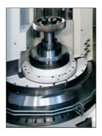
grinding external spur and helical gears up to 10 mm with an outside diameter of maximum 500 mm and gear width up to 520 mm. The machine is suitable for single- or twin-spindle dresser use, and automation options are available. The gear center has a multi-station turntable and twin-spindle dresser, so different tooling concepts can be used, such as dressable and non-dressable ceramic tools for prototype machining and grinding of medium- to high-volume series.
