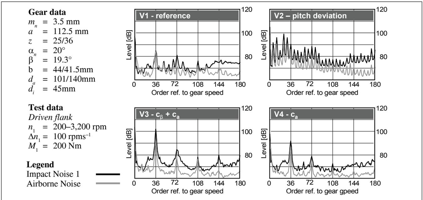
Figure 7—Fourier analysis of impact and airborne noise.
