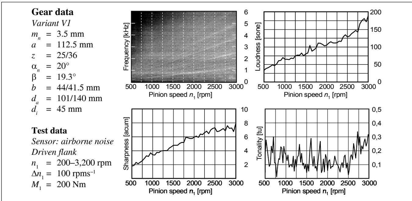
Figure 6—Noise analysis of a speed ramp.
